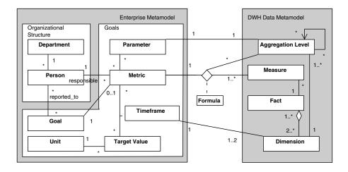
Figure 6. Weaving Model connecting the Goal Model (left) with the Data Model (right). Only a part of the Enterprise Model is shown here for readability. It has more than the two aspects, and the organizational aspects has more than the two elements shown here.
